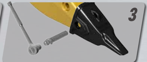
Insert Helical Pin & Rotate 180 degrees with Socket Wrench to Engage Lock
