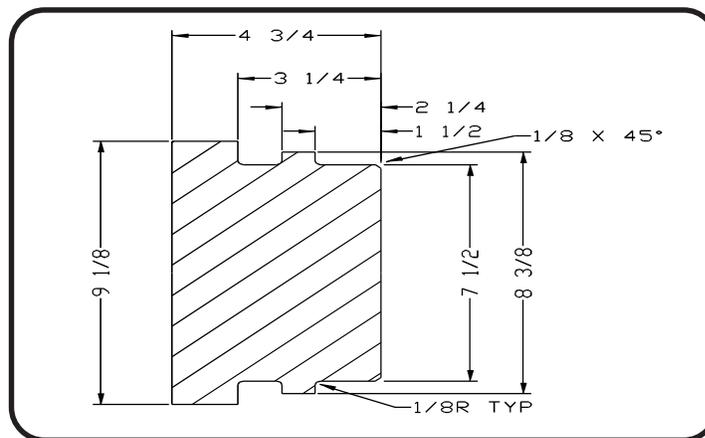
P125/P125HD Bearing Spacer/Press Plate
