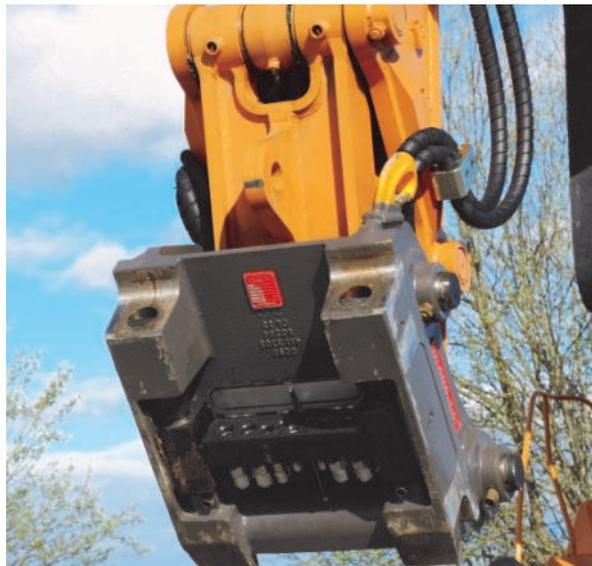
OilQuick is an automatic quick coupler system for excavators, which allows hydraulic work tools to be connected and disconnected from the drivers cab.
