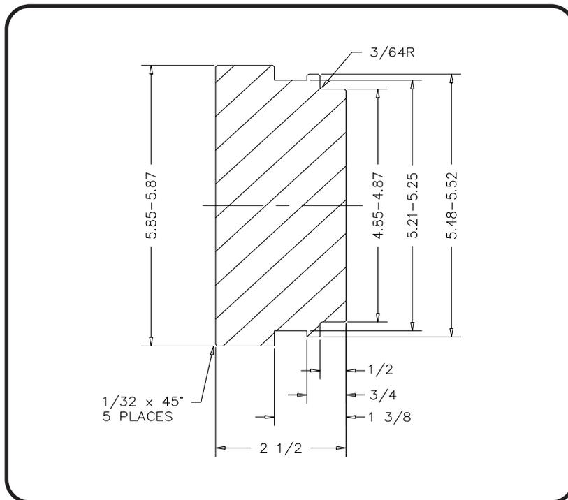
*N80 Bearing Spacer/Press Plate
