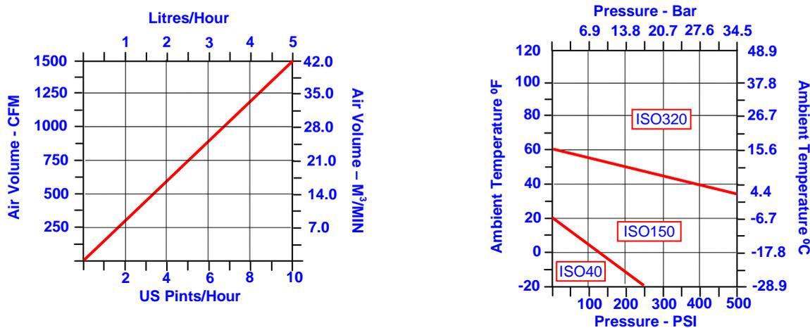
At low temperatures of 5°C (41°F), and in hot humid conditions with higher air pressures, when hammers can freeze up. Anti-freeze additive may be required at a rate of 1-2 litres (2-4 pints) per hour or more as necessary.
