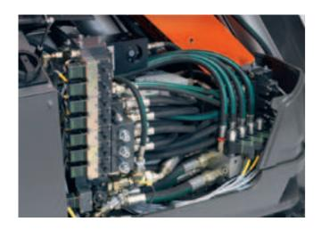
On the side of the machine is a door. Inside is everything you need to manage filters, electric components, oil or troubleshooting. There are also hydraulic hoses with plugin connections, for easier hose changes.
